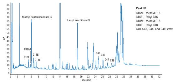
Figure 2. Chromatogram of an olive oil labeled as extra virgin, showing good resolution of critical ethyl and methyl esters.
