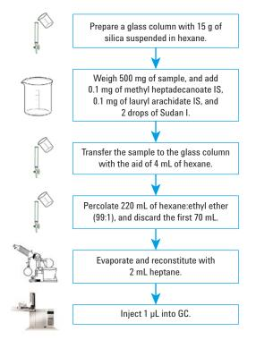
Figure 1. Workflow to prepare olive oil samples for GC analysis according to the IOC.
