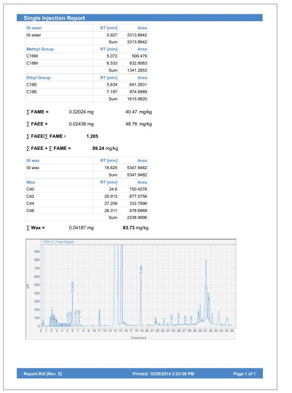
Figure 3. Example of a report created by Agilent OpenLAB Data Analysis Intelligent Reporter, showing the fatty acid methyl and ester content and ratios in a sample of olive oil.
