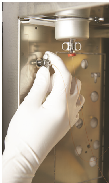
Figure 3. Agilent self-tightening column nuts installed at the transfer line and inlet fittings.
