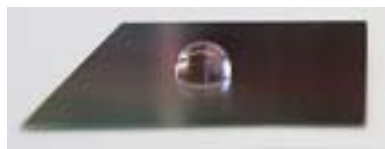
Figure 3. Water droplet on an UltiMetal Plus-treated stainless steel surface.
