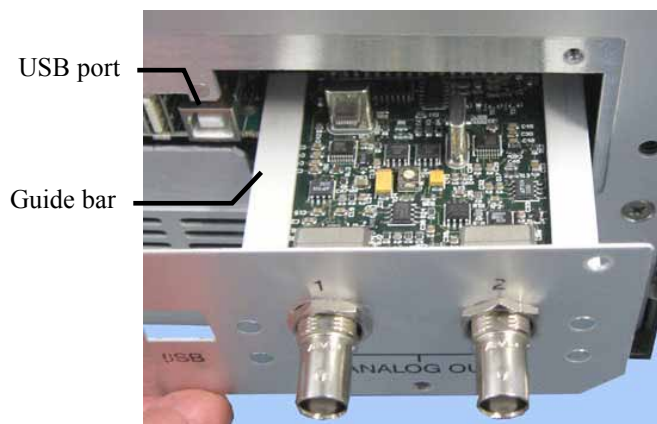
Fig. 10: Installing the DAC board
