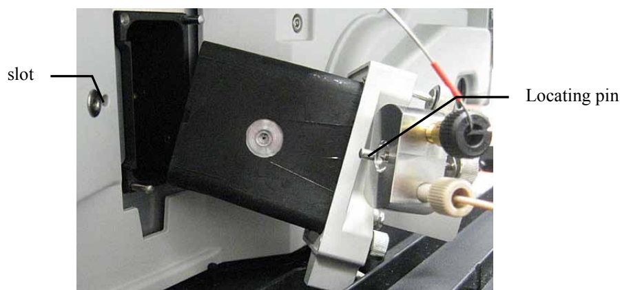
Fig. 37: Installing a flow cell with adapter block (here semi-micro flow cell)
