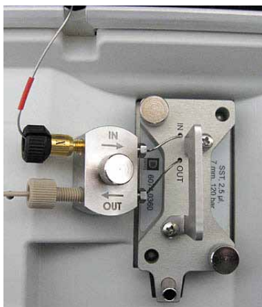
Fig. 38: Analytical flow cell with stainless steel inlet capillary (here: Viper capillary)
