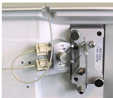
Fig. 39: Analytical flow cell with PEEK inlet capillary
