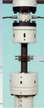
Axial-force/torsion compound detector Detector for torsional displacement angle between gauge marks
