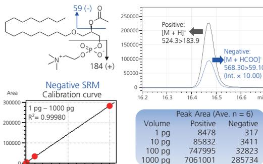
Fig. 4 Optimization of MRM Parameters for PAF
