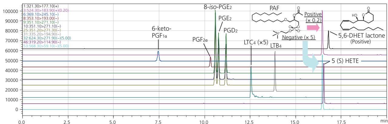
Fig. 5 Simultaneous detection of 10 compounds (100 pg each)
