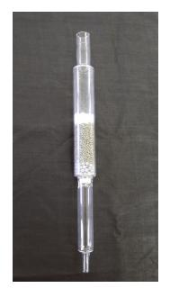
Fig. 1 High-Salt Sample Combustion Tube
