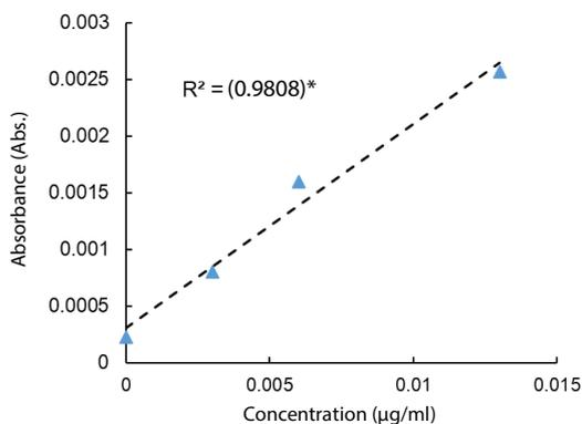
**Fig. 3 Calibration Curve of Low Concentration Region (UV-2600i)**
