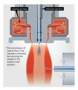
Figure 3. Heated ESI probe
