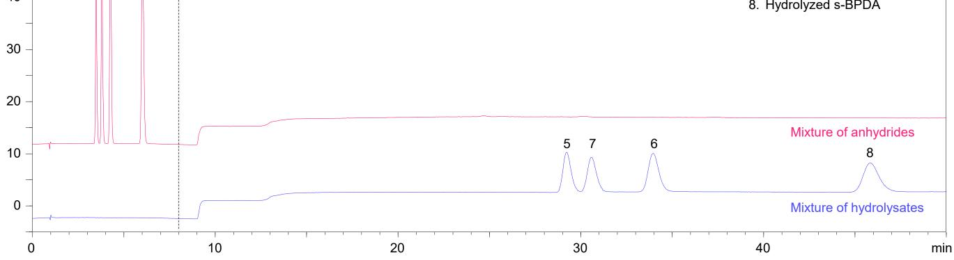
Figure 5: Chromatograms of carboxylic anhydrides (top) and hydrolysates (bottom)
