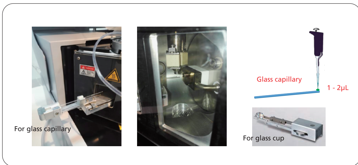
Figure 2 Injection mode for DCBI analysis (LCMS-8040)
