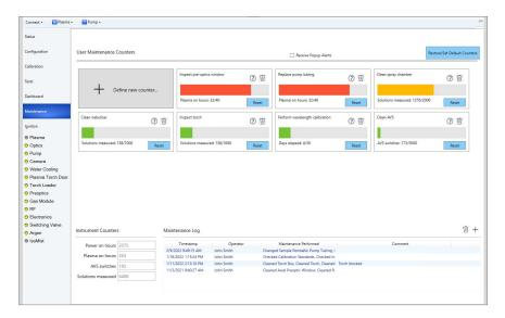
Alerts address common reasons for service calls, such as poor precision due to worn pump tubes, or poor sensitivity due to a dirty pre optic window. By alerting the analyst of a problem and then guiding them through the process of fixing it, the expense and downtime of a service call can be avoided.
