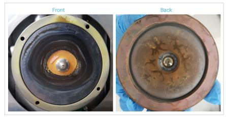
The standard platinum-tipped sampler cone (without nickel plating) after 1,090 hours of run time with a 10% aqua regia matrix. This demonstrates the copper base corrosion problem. Black coating is copper oxide and surrounding the tip the copper is worn away.
