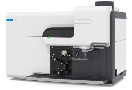
The 4210 MP-AES uses only nitrogen as a fuel, eliminating combustible gas usage and gas transportation. With minimal standby power consumption you can use less gas and electricity, compared to comparable techniques for crude and residual fuel analysis.
