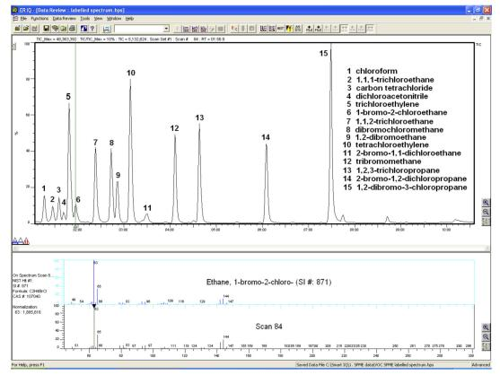
Column: Rtx-1MS (15 m x .25 mm x 1.0 μm) Column temperature program: 60 °C held for 1.0 minute, ramp at 6 °C/min. to 80 °C, ramp at 12 °C/min. to 120 °C, ramp at 20 °C to 180 °C.
