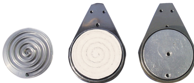
Figure 1. TOPAS badge: basic aluminium body with cut groove (left), badge fitted for measuring, filled with Tenax and encapsulated with the microporous Teflon membrane (middle) and reverse view of badge fitted for storage and GC analysis; view of desorption gas inlet and outlet (right).
