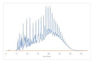
Fig 3. Overlay of Reference Gas Oil Sample with CS Blank
