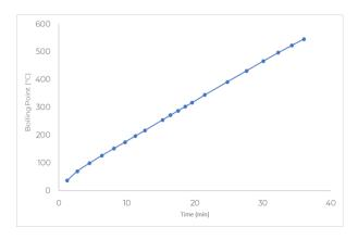
Fig 2. C5-C44 n-Paraffins RT vs Boiling Point Calibration
