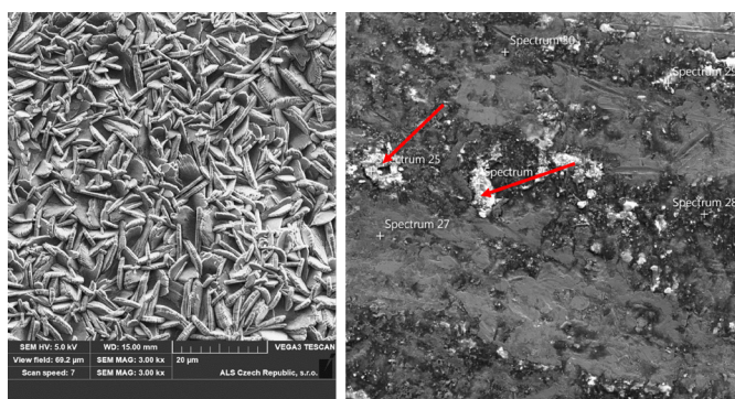
Figure 2: (A) anti-corrosive layer; (B) corrosion traces
