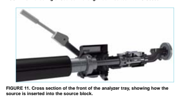
FIGURE 11. Cross section of the front of the analyzer tray, showing how the source is inserted into the source block.
