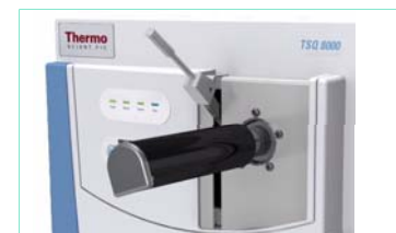
FIGURE 10. Rendering of Source Exchange Tool inserted into TSO 8000.
