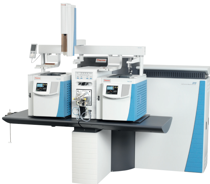
Figure 1. Thermo Scientific DFS Magnetic Sector GC-HRMS.
