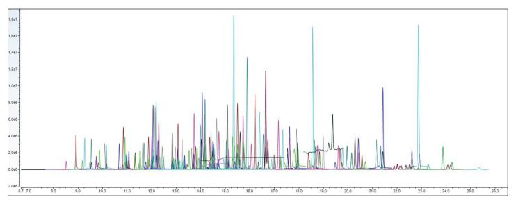
Figure 1. Timed SRM acquisition for analysis of 200+ pesticides at 50 ppb in a single run on the TSQ 9610 GC-MS/MS system
