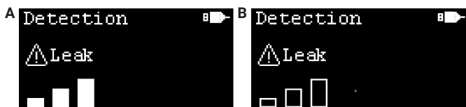
Figure 7. Examples of gas leak for gases with higher thermal conductivity than air (A) and gas leak for gases with lower thermal conductivity than air (B).
