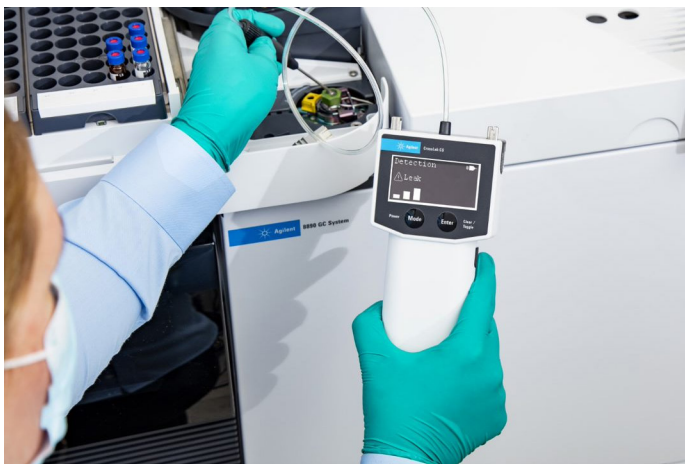
Figure 12. Leak checking the GC inlet septum nut with the Agilent CrossLab CS Electronic Leak Detector.
