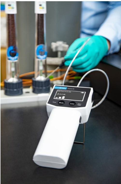
Figure 8. Example of leak checking a Gas Clean filter unit with the Agilent CrossLab CS Electronic Leak Detector.
