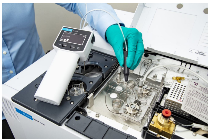
Figure 6. Example of leak checking a valve system with the Agilent CrossLab CS Electronic Leak Detector.
