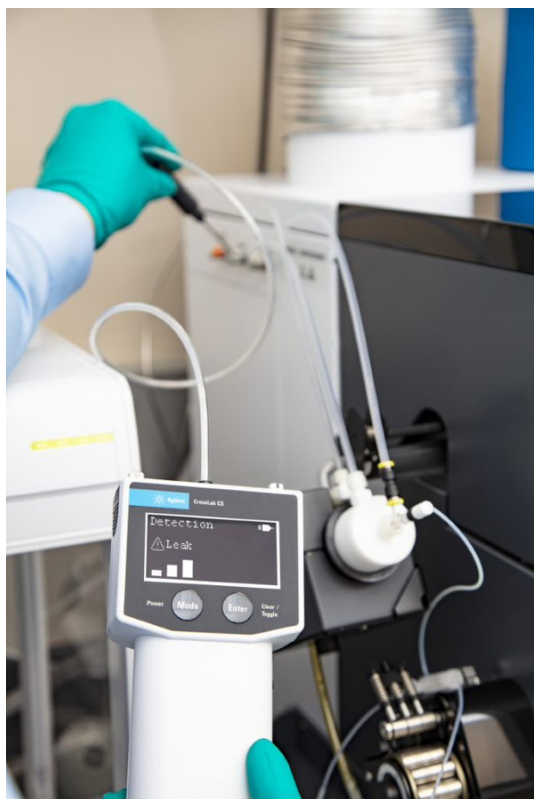
Figure 18. Using the Agilent CrossLab CS Electronic Leak Detector to check for leaks at the option gas port on the Agilent 7900 ICP-MS.
