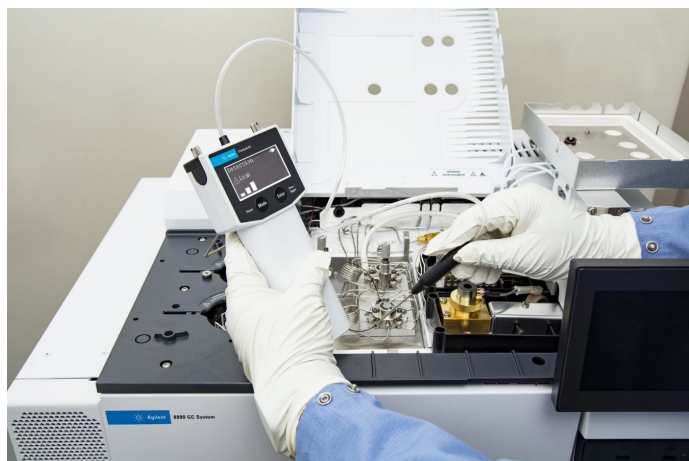
Figure 15. Using the Agilent CrossLab CS Electronic Leak Detector to check for leaks at connections in a valved GC system.
