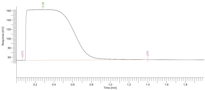
Figure 5. FID Signal, calibration run with 0.3µL ethanol added to a 330 mL empty and blank can.
