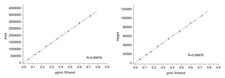
**Figure 6.** Calibration of the FID with liquid injection of ethanol in an empty and blank calibration can. Liquid injections varied between 0.02 to 0.3  $\mu$ L, can volume was 330 mL. The shown error bars result from 2 injections at each level.
