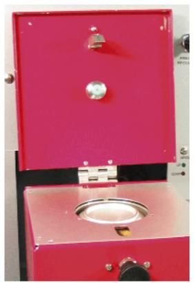
**Figure 3.** QCS 1 - Sample Oven for beverage cans. The picture shows the open oven with a beverage can inserted bottom-up. In the middle of the open ovenlid a septum screw is seen. This septum screw presses the septum onto the convex bottom of the beverage can. Because of the conical shape the septum fits all type of beverage cans or other solid vessels. The extra hardened headspace needle penetrates the septum and the metal bottom of the can.
