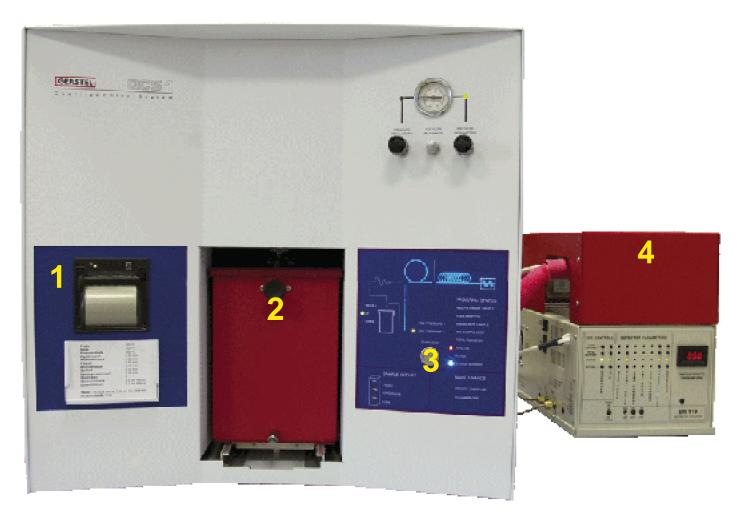
**Figure 1.** Quality Control System QCS 1 – Headspace Sampling System for beverage cans, in this configuration equipped with a Flame Ionization Detector FID; 1 optional printer, 2 sample oven, 3 control panel, 4 optional FID.
