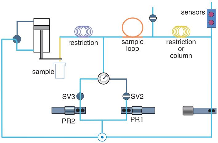
Figure 2. QCS 1- flow diagram of the valveless headspace sampling technique.
