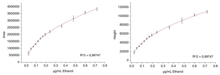
**Figure 8.** Calibration of the Sensor with liquid injection of ethanol in an empty and blank calibration can. Liquid injections varied between 0.01 to 0.3  $\mu$ L, can volume was 330 mL. The shown error bars result from 3 injections at each level.
