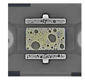
Top: Cross-Sectional Image Scanning Region = 9 mm Bottom: Area Ratio Measurement (Imaging with PCT)
