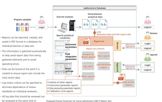
Proposed Process Flowchart for Using LabSolutions DB/CS Report Sets
