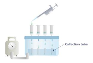
Warming the collection tubes in a water bath at 60 to 65 °C, dry the solution collected in the collection tubes by using a nitrogen purge. (11.5)
