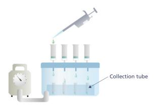
Warming the collection tubes in a water bath at 55 to 60 °C, dry the solution collected in the collection tubes by using a nitrogen purge. (11.4.6)
