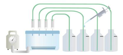
Stop the vacuum, open the manifold lid, remove the reservoir, and insert the collection tubes. Place 5 mL of ammonium hydroxide methanol solution in the bottles. Adjust the output of the vacuum pump so that the ammonium hydroxide methanol solution passes through slowly. Add another 5 mL of the same solution and pass it through. (11.4.5)
