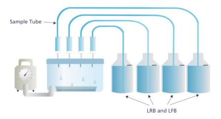
When the sample is depleted, add 10 mL of 1 g/L ammonium acetate to each sample bottle to wash them, and then add 1 mL of methanol. Dry the cartridges at high vacuum for 5 minutes. (11.4.3, 11.4.4)
