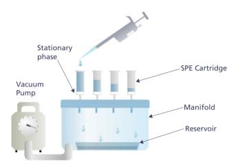
Connect the sample introduction tubes and then start the vacuum operation. Adjust the output of the vacuum pump so that the flow rate is 5 mL/min. (11.4.2)
