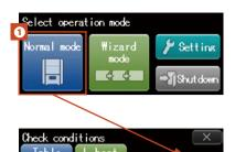
After system startup, press (1) and then (2) to start deposition.
