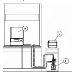
Please prepare for the draft chamber at the inside dimension of more than D650 × W1000 × H60 (mm). Sirrocco fan: CES-V
