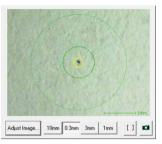
Sample Image at an Irradiation Diameter of 0.3 mm (Extended Zoom) Sample: stainless powder (approx. 0.1 mm) collected on filter paper
