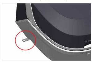
Note: When preparing for slippage or falling due to an earthquake, etc., install presser brackets on the equipment legs and take anti-earthquake measures on the installation table itself.
