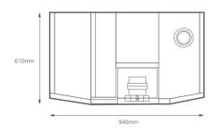
AA-7800/AAC Dual Atomizer System Dimensions (Top surface)
