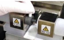
Replacing the Graphite Tube
