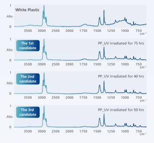
to deteriorate, and it is evident that the shape of the infrared spectrum has changed.
