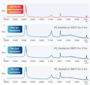
The measurement of a light brown semi-transparent contaminant on a plated item was performed. The figure above shows that the spectral pattern of the acquired infrared spectrum differs from the standard polyethylene (PE). Plastic Analyzer shows the best match is heated PE. The Thermal-Damaged Library makes it useful for surmising the thermal history of the plastic.
