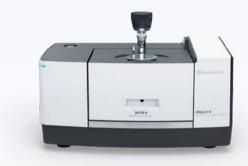
When analyzing plastics, libraries are used to qualify their material properties. However, infrared spectra of plastics that have degraded due to heat or UV rays differ in shape from standard spectra, and qualifying them can sometimes be difficult. To address this, the Plastic Analyzer includes a deterioration library, so highly accurate qualification can be performed reflecting the state of deterioration.
