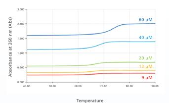
Melting Curve of Nucleic Acid (M13 Primer)
