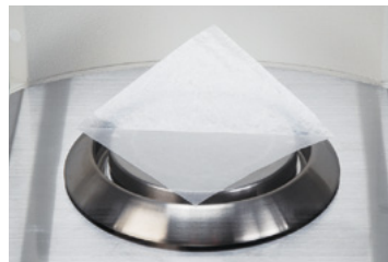
Numerical values do not stabilize due to electrically charged weighing paper
