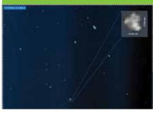
**Step 4.** Each spectrum is then compared against a spectral library to identify the chemical composition of each particle. The LDIR has a high-magnification visible camera to photograph particles. In this case, a polystryene microplastic particle, identified in sewerage.
