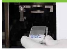
**Step 3.** The instrument will scan an area using light of a single wavenumber to locate all the particles. It takes only 4 minutes to scan an area 10 x 10 mm at 5 µm pixel size. The instrument then targets the identified particles (appearing as bright spots) and collects an IR spectrum of each one.
