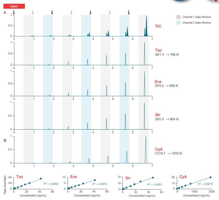
Clinical research assay for quantification of immunosuppressant drugs Tacrolimus (Tac), Everolimus (Eve), Sirolimus (Sir), and Cyclosporin A (CyA) in whole blood using the Transcend LX-2 system interfaced to a Thermo Scientific<sup>™</sup> TSQ Quantis<sup>™</sup> triple quadrupole mass spectrometer. Seven injections on 2 parallel UHPLC channels (A) were used to generate calibration curves (B) for each of the four drugs.
