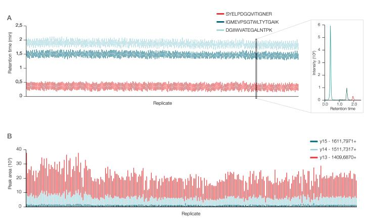
Retention time (A) and peak area (B) reproducibility of a high-throughput targeted proteomics assay for quantifying SARS-CoV-2 peptides in clinical research samples across 5 days. The Transcend TLX-4 UHPLC system was utilized for on-line sample clean-up and analysis of 500 respiratory tract swab samples per day.
