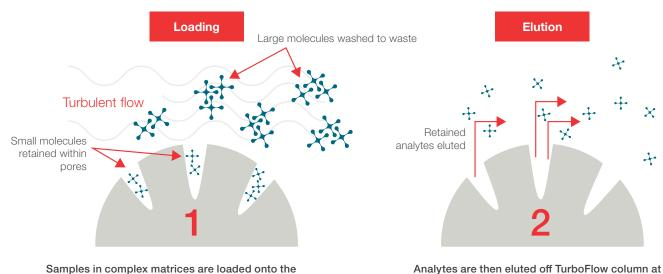
Samples in complex matrices are loaded onto the TurboFlow column at high velocity, leading to biased diffusion of small molecules into column pores. Within pores, analytes are retained on the stationary phase— RP, IEX, and mixed mode available.
