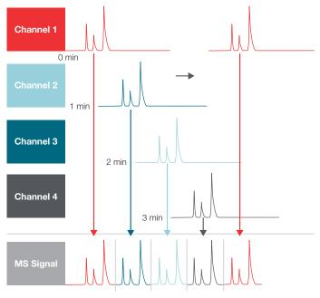
Injections are interleaved to maximize throughput and mass spectrometer utilization.
