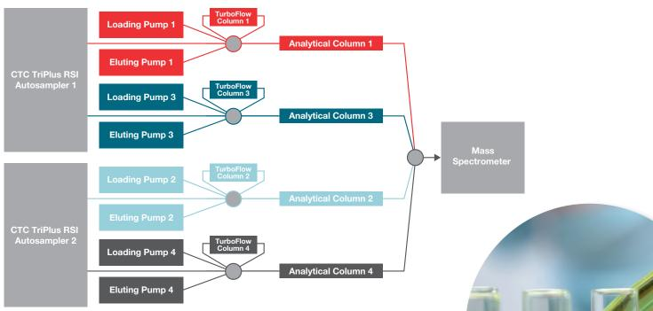
Diagram of Transcend TLX-4 system with four independent flow paths.
