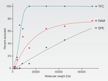
TurboFlow technology offers superior sample cleanup to restricted access media (RAM) and solid phase extraction (SPE).
