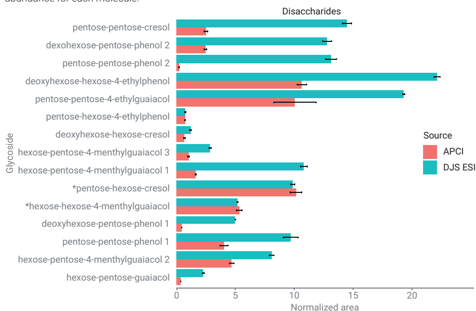
Figure 5. A comparison of the Dual Jet Spray ESI and APCI LC/MS sources. Source settings were optimized for the highest abundance for disaccharides. In every case, ESI had the same or higher abundance for each molecule.
