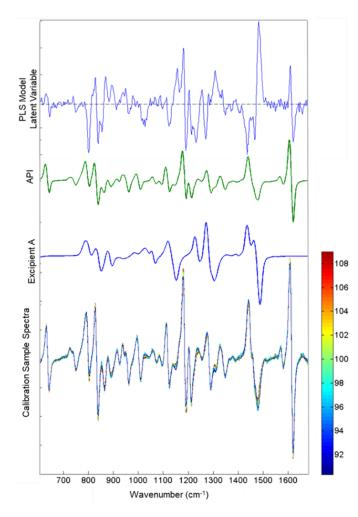
Figure 4. From bottom to top: calibration spectra colored according to API concentration  $1^{st}$  derivative SNV, excipient A, API  $1^{st}$  derivative SNV, and PLS model latent variable 1.
