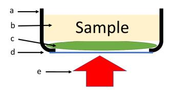
Figure 2. Schematic of sample setup. a) Agilent TRS100 tray, b) liquid sample, c) empty capsule, d) clear tape, e) laser of the Agilent TRS100.
