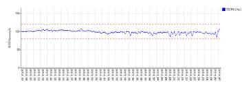
Figure 1. ISTD recovery of sample analysis over 10 hours using the Agilent 7900 ICP-MS.
