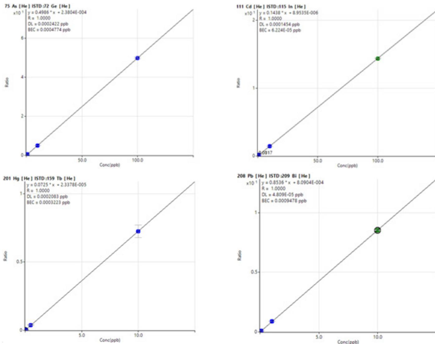
**Figure 3.** Representative calibration curves for As, Cd, Hg, and Pb, showing extremely low, sub-ppt instrument DLs and good linearity ( $R = 1.0000$ ) across the calibration range.
