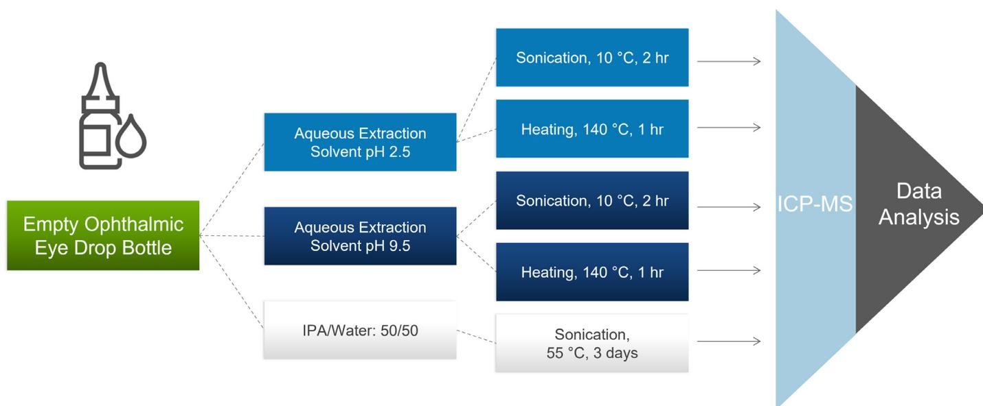
**Figure 2.** The analytical workflow used to extract elemental impurities from empty plastic ophthalmic eye drop bottles for determination using ICP-MS.
