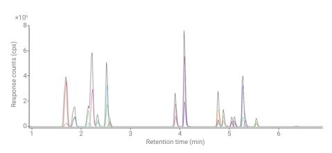
Figure 1. MRM overlay of 18 alkaloids from different classes at a level of 50  $\mu$ g/L for each.
