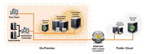
Figure 6. Chromeleon CDS Hybrid Cloud Deployment Example
