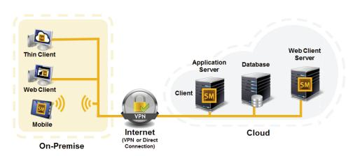
Figure 5. SampleManager LIMS Cloud Deployment Example
