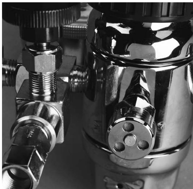
Figure J. Conventional (left) and Hydrogen Pressure Relief Valves
