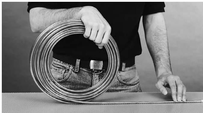
Figure H. Uncoil Tubing without Creating Bends
