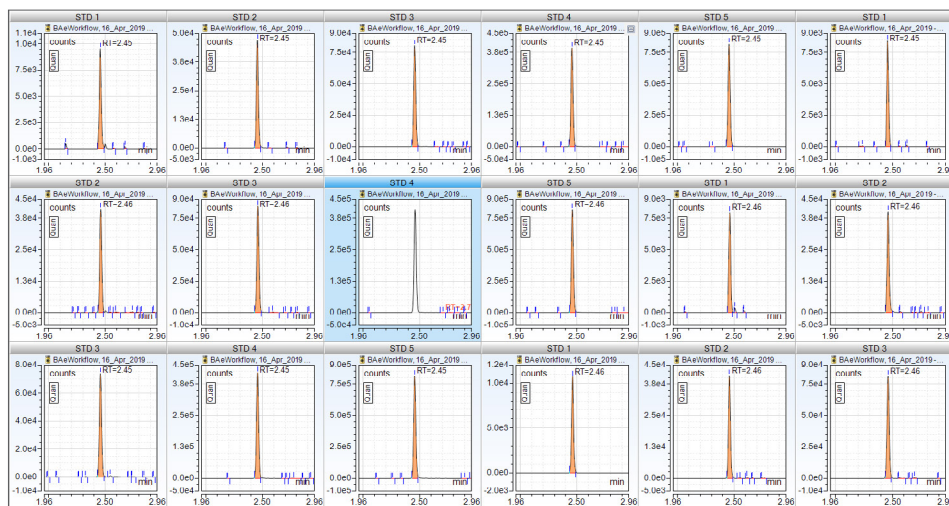
Figure 7. Calibration standard quantitation ions across a sequence for a specific component per injection
