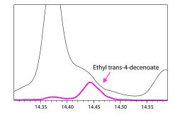
Fig. 5 Mass Chromatogram and TIC of Ethyl Trans-4-Decenoate
