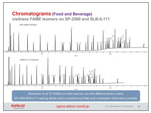
Trans fat content is reported on nutritional facts panels as part of proper food labeling. It is desirable to use a column which can resolve trans FAME isomers from cis FAME isomers, so trans fat values are not biased high. These chromatograms of C4 to C24 FAMEs on the SP-2560 and SLB-IL111 represent the ultimate in cis/trans FAME analysis. This is because the SP-2560/SLB-IL111 pairing allows the most comprehensive fatty acid composition information possible.
