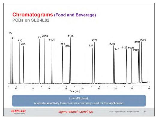
Polychlorinated biphenyls (PCBs), classified as persistent organic pollutants (POPs), have been found in several food types, such as milk. This chromatogram of 19 PCBs was analyzed on the SLB-IL82. In addition to the low level of MS bleed, the SLB-IL82 offers alternate selectivity than the columns commonly used for this application.
