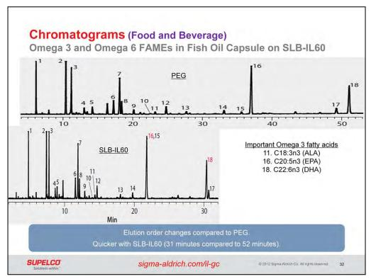
Fish oil capsules are taken to gain the benefits associated with omega 3 fatty acids. This sample is very similar to the menhaden oil sample shown on the previous slide. Shown are chromatograms generate with a column made with polyethylene glycol (PEG) phase and an SLB-IL60. The SLB-IL60 analysis resulted in two elution order changes. Additionally, the analysis was quicker (31 minutes compared to 52 minutes).
