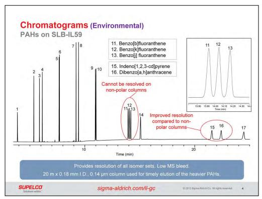
Polycyclic aromatic hydrocarbons (PAHs) are produced as by-products of burning fuel. Several PAHs are identified as carcinogens. The PAHs of interest include several isomer sets. This chromatogram of 19 PAHs on the SLB-IL59 highlights the ability of this column to provide resolution of all isomer sets, and exhibit low MS bleed. A 20 m x 0.18 mm I.D., 0.14 µm column was used for the timely elution of the heavier PAHs.
