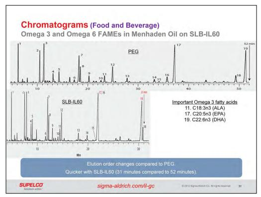
Menhaden oil contains an abundance of omega 3 fatty acids. This slide compares chromatograms from a column made with polyethylene glycol (PEG) phase to an SLB-IL60. The SLB-IL60 analysis resulted in two elution order changes. Additionally, the analysis was quicker (31 minutes compared to 52 minutes).
