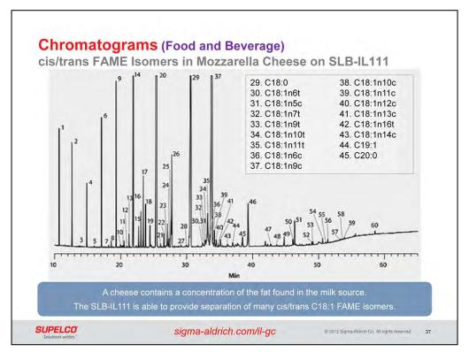
A cheese contains a concentration of the fat found in the milk source. This is because almost all of milk's nutrients are retained during the process of manufacturing cheese. This chromatogram shows the analysis of fatty acids (as fatty acid methyl esters) extracted from a mozzarella cheese made with buffalo milk. The SLB-IL111 is able to provide separation of many cis/trans C18:1 FAME isomers.
