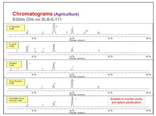
Each pure edible oil has a unique combination of FAMEs in specific ratios. Therefore, GC fingerprinting can be used to monitor purity. It can also be used to detect adulteration when a cheaper, inferior oil is added to boost the volume of a premium, higher priced oil. The SLB-IL111 column is able to provide the necessary resolution of key FAME isomers found in several edible oils for effective fingerprinting.
