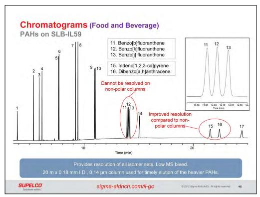
Polycyclic aromatic hydrocarbons (PAHs) are produced as by-products of cooking meat at high temperatures. Several PAHs are identified as carcinogens. The PAHs of interest include several isomer sets. This chromatogram of 19 PAHs on the SLB-IL59 highlights the ability of this column to provide resolution of all isomer sets, and exhibit low MS bleed. A 20 m x 0.18 mm I.D., 0.14 µm column was used for the timely elution of the heavier PAHs.
