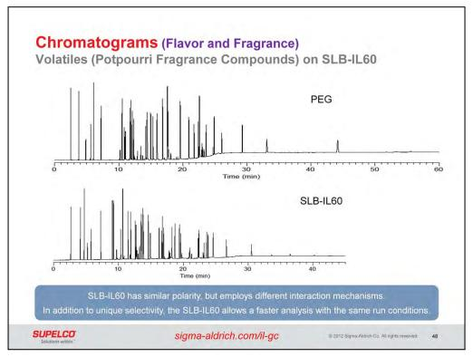
Columns made with polyethylene glycol (PEG) phases are commonly used for fragrance compounds. This slide shows the analysis of a mixture of fragrance compounds on a PEG and also on a SLB-IL60. The SLB-IL60 has similar polarity, but employs different interaction mechanisms. In addition to unique selectivity, the SLB-IL60 allows a faster analysis with the same run conditions.
