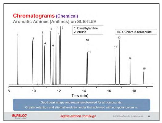
This chromatogram of an aromatic amines mix was generated using an SLB-IL59 ionic liquid column with FID detection. Analytes range in size from aniline (peak 2) to 4-chloro-2-nitroaniline (peak 15). Good peak shape and response was observed for all compounds. Compared to a non-polar column, retention of analytes was greater, and elution order was markedly different.
