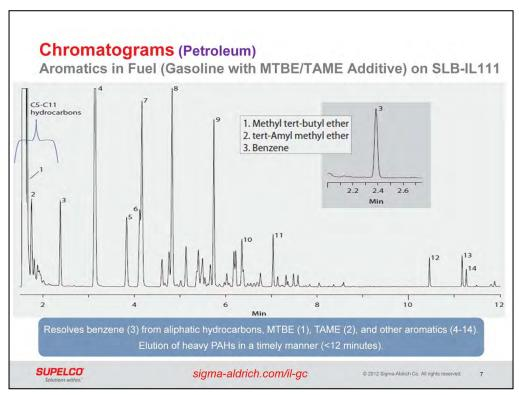
This chromatogram is of reformulated gasoline with MTBE and TAME as oxygenates. A 30 m SLB-IL111 column was able to provide the resolution of benzene from all other components. Also note that the heavy constituents (methylnaphthalenes, peaks 13 and 14) elute in a timely manner with great peak shapes.
