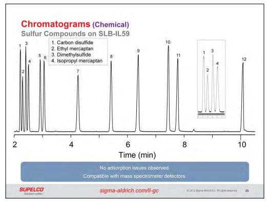
lonic liquid columns can also be used for the analysis of sulfur compounds. This chromatogram shows the analysis of 12 sulfur compounds on the SLB-IL59 column using a mass spectrometer for detection. Analytes include carbon disulfide (peak 1) to diethyl disulfide (peak 12). No adsorption issues were observed. The inset shows the separation of the first four analytes.
