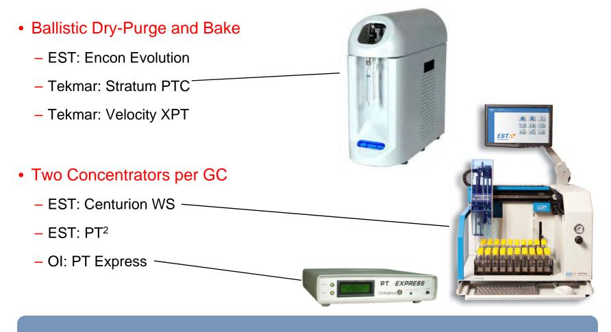
Example equipment that allows P&T to catch up with improvements in GC speed.
