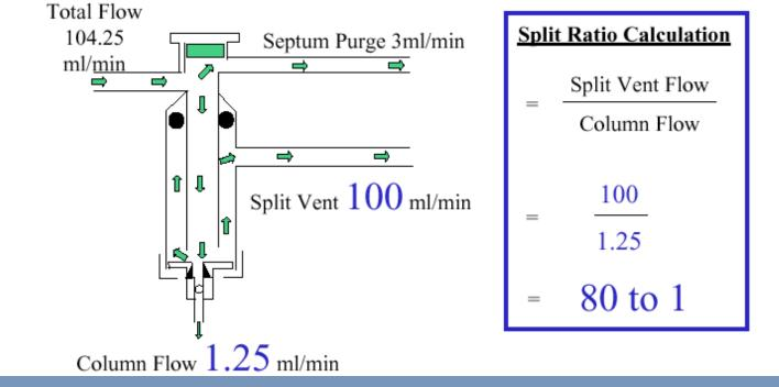
Split ratios range from <5:1 (wide bore column applications) to >400:1 (Fast GC applications). User should experimentally determine which split ratio works best for their application.
