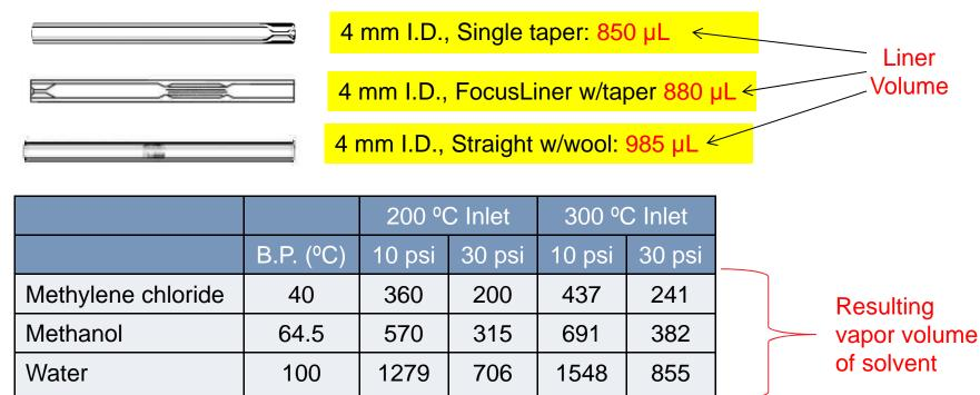
Use an inlet liner with an internal volume equal to or larger than the expansion volume of the solvent.
