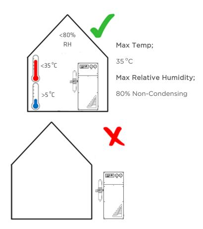
Generator MUST NOT be stored or installed outside.
