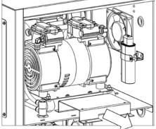
Figure 1: Transit Bracket Removal
