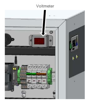
Figure 4: Voltmeter Location
